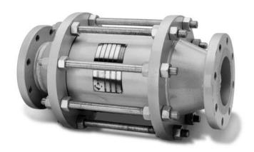
Designed with flanged connections, this Arrestor provides the option of the removal of the flame cell element for easy cleaning and replacement without disconnecting of the pipe connection. Standard housing construction is carbon steel and stainless steel. The element is available in stainless steel. Special material and protective coatings are available on request.
